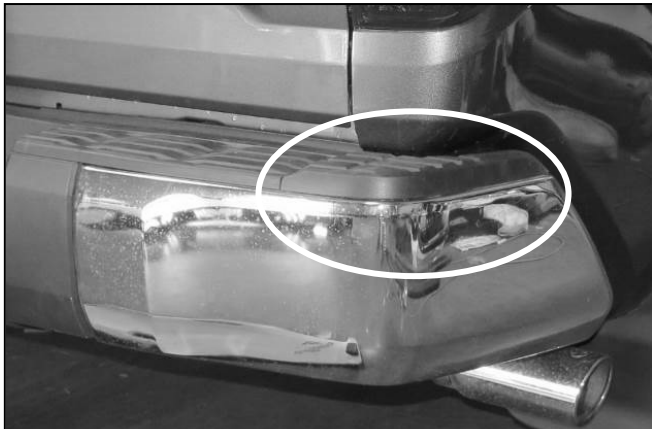
(Fig 3) Use a flat blade screwdriver to pry the plastic cover from the top of edges of the bumper
