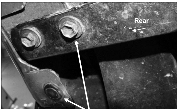
(Fig 5) Remove Factory Hardware and Plastic Clip from the underside of the bumper
